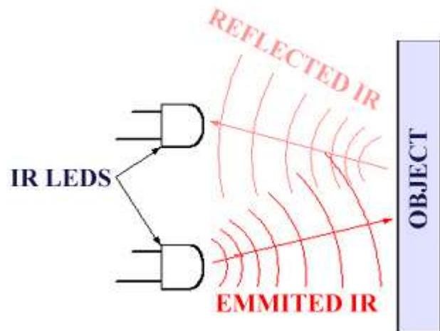
The physics which govern reflection of visible and infrared light are the same. IR LED's are easily available, and so are the sensors to detect IR radiation.
