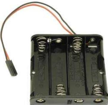
Consider buying or salvaging a battery holder from a gadget like an old toy car. They are helpful and neat! Check for sizes and shapes though, as 9v batteries are sometimes more useful than 'AA' sized ones and may have higher current ratings.
