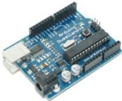
We assume you are using the Arduino Duemilanovae, which should be directly compatible with Decimila and UNO. If you have any other version or clone, do ask for guidance on the Arduino forums.
